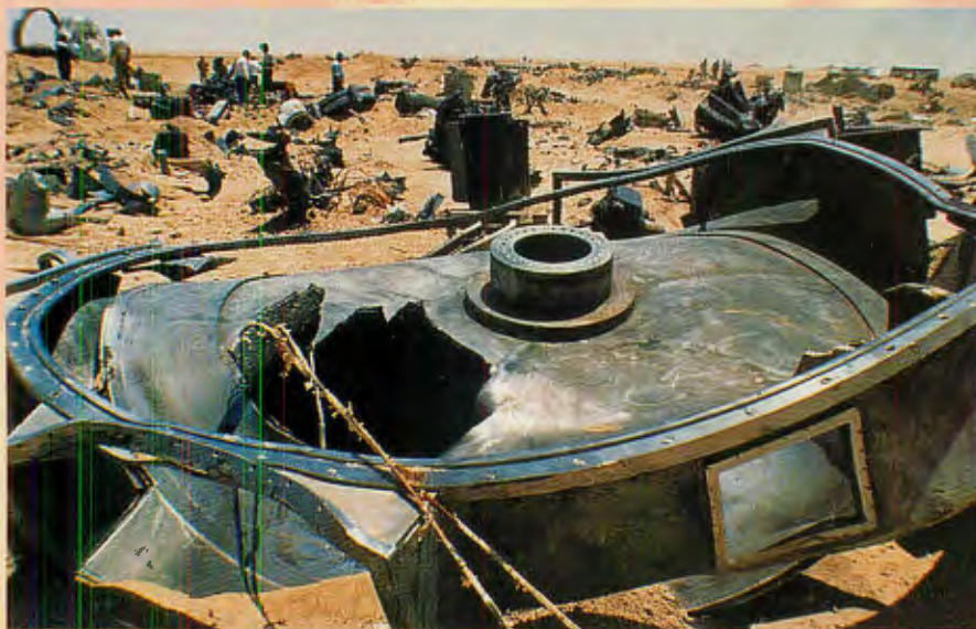
Calutrons for uranium enrichment were unilaterally destroyed by Iraq. Uranium enrichment is a major concern of United Nations weapons inspectors, as it's been a key element in Iraq's quest to build an atom bomb.
